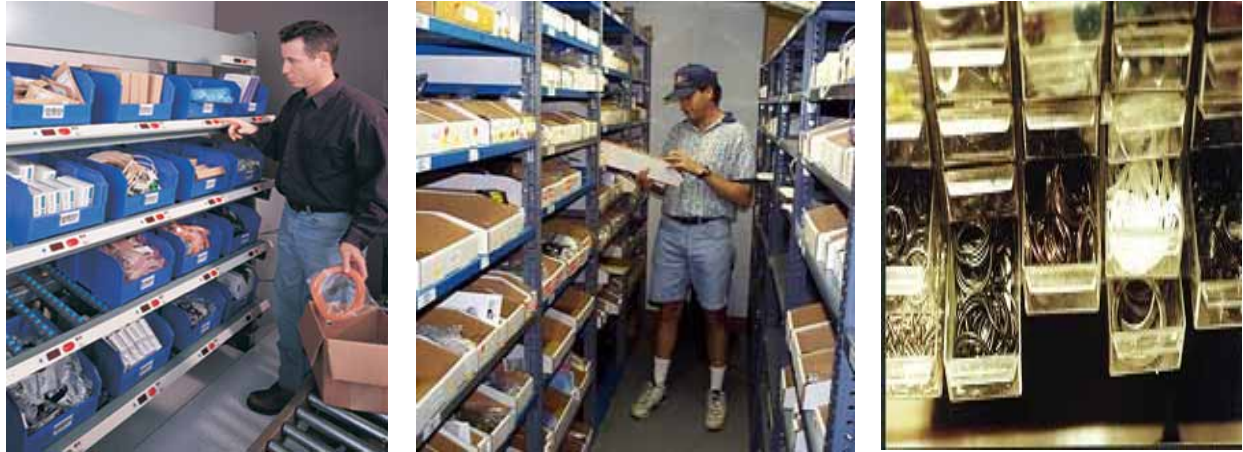
Figure 6 – Spare Parts in Case Flow Rack, Shelves, and Bin Drawers
