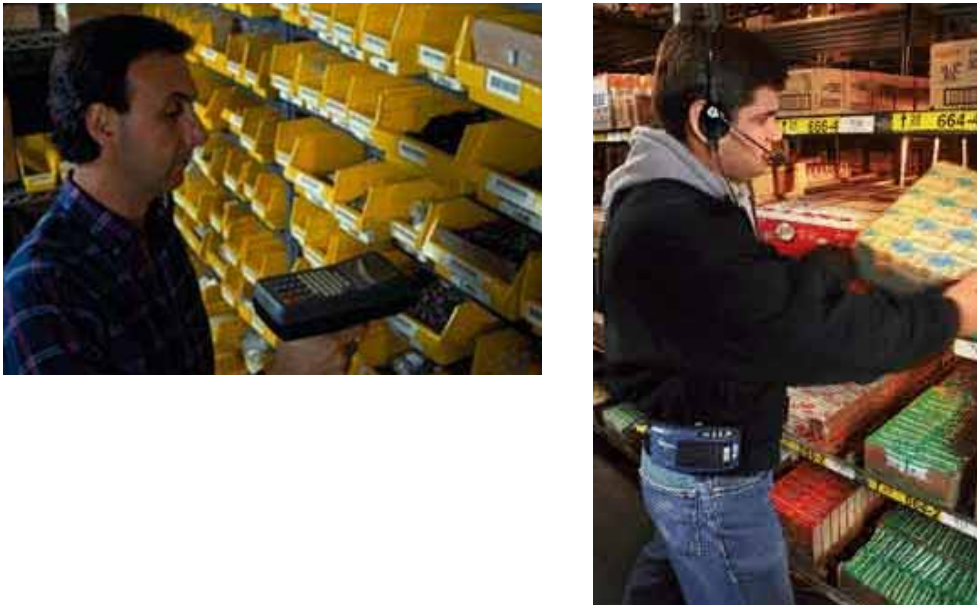
Figure 7 – RF Handheld Scanner and Voice Directed Parts Selection
